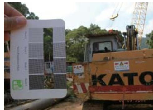
*The Ringelmann chart is used to monitor the exhaust of on-site machines
