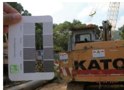
*The Ringelmann chart is used to monitor the exhaust of on-site machines
